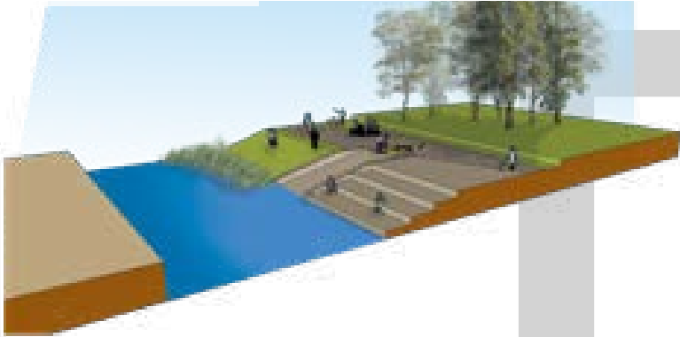
Figure 130. | river edges with soft sloping edges, gabion construction slip access and steps
